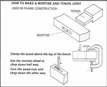
The Mortise Chisel is used to cut the mortise in a Mortise and Tenon Joint the Chisel has a heavy rectangular blade and metal ferrules around the handle to prevent the handle splitting when it is hit with a mallet.
