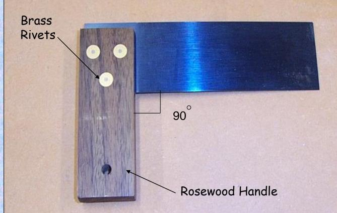
The Try Square is used for marking a line at right angles to an edge
