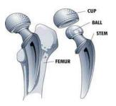
The materials used to make artificial hip joints must be resistant to corrosion, degradation and wear. They must also have similar mechanical properties to bone. For example, the materials must be strong enough to take the person's weight and must be able to bear stress without fracturing.
